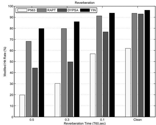
Figure 4: Pitch estimation in a reverberant room of length 5m, width 4m, height 3m. Reverberation time (x-axis)  $T_{60}=0.5$  s (left) to clean speech in a non-reverberant room (right). Performance metric is the modified hit rate (y-axis) given as a percentage of overall hits.
